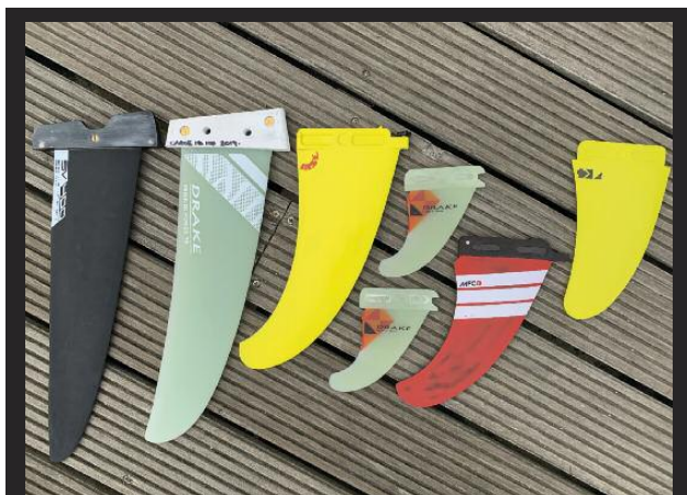
A range of fin types and shapes: (from left to right): slalom/race, freeride, freewave single, freewave thruster setup (tri fins) and freestyle
