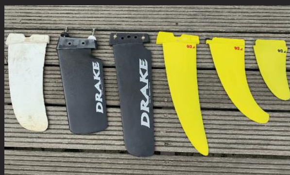
Plastic progression: (from left to right) Hifly older-style intermediate, Drake Shallow beginner (two lengths), K4 freeride/freewave single/freestyle
