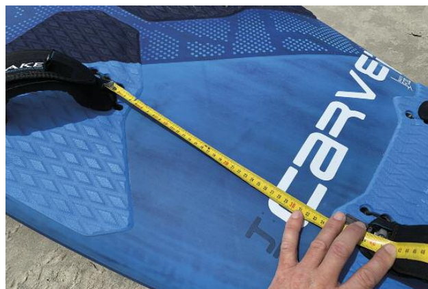
Measure the spread between the back screw of the front strap and the front screw of the back strap on the same side
