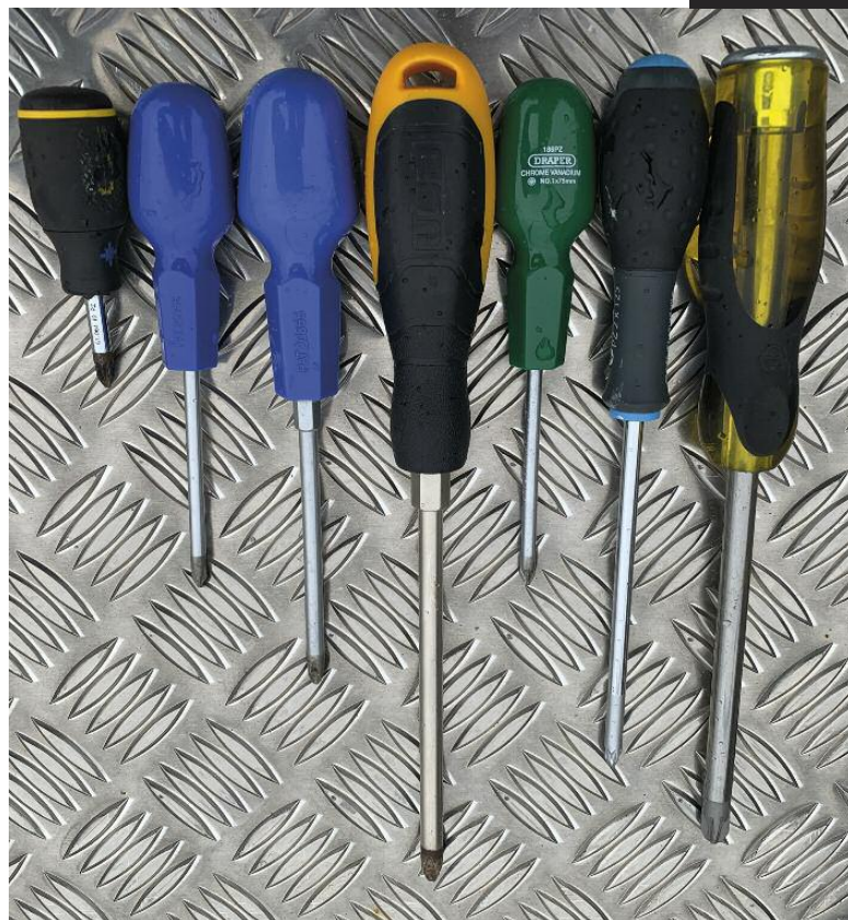
Seven similar screwdrivers but only the middle one is good for most footstraps
