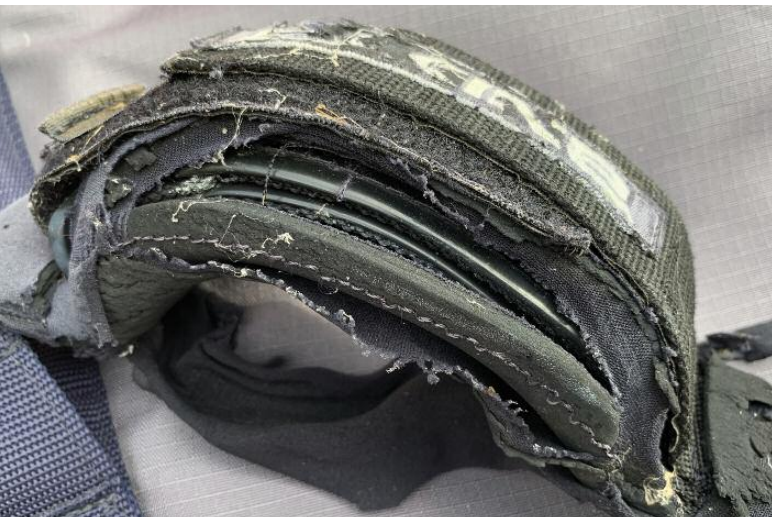
Replace long before the footstrap degrades into more layers than a Viennetta!
